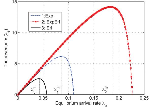
Fig. 7. The revenue vs. equilibrium arrival rate  $\lambda_e$  in three examples with the parameters:  $R=100, C=1, \beta=2, \mu_Y=1.2$  and  $\mu_X=0.5$ ; (1) the channel follows the ExpErl case; (2) the channel follows the Erl case; (3) the channel follows the Erl case.
