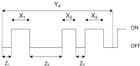
Fig. 3. A sample ON-OFF process with a realization of an effective service time  $Y_e$  where the PUs' channel at state OFF will continue being OFF for an additional time  $Z_1, Z_2$  and  $Z_3$  before changing to state ON.  $X_1, X_2$  and  $X_3$  are corresponding ON periods, respectively.
