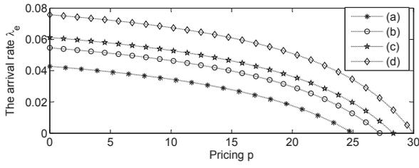
Fig. 5. SU customer individual arrival rate  $\lambda_e$  vs. pricing  $p$  with  $R=40, C=1$  and the Erl channel in four case: (a)  $\beta=2, \mu_Y=1.2$  and  $\mu_X=0.5$ ; (b)  $\beta=2, \mu_Y=1.2$  and  $\mu_X=0.6$ ; (c)  $\beta=1.5, \mu_Y=1.2$  and  $\mu_X=0.5$ ; (d)  $\beta=1.5, \mu_Y=1.2$  and  $\mu_X=0.6$ .
