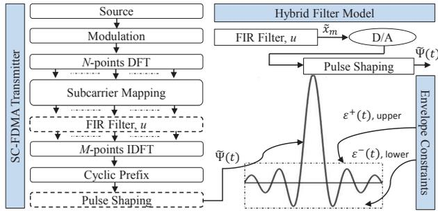
Fig. 1. Hybrid filter for SC-IFDMA Transmitter
